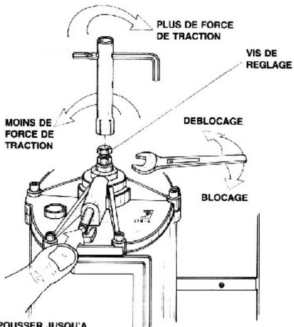
**POUSSER JUSQU'A L'ENCLÈCHEMENT ET TOURNANT L'ARBRE AVEC LA CLE**
